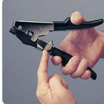
**Tensioning Adjustment Knob and Automatic Cut-Off Mechanism:** Turn adjustment knob clockwise to increase tension and counter clockwise to decrease tension. **CAUTION:** Do not over tighten adjustment knob with fingers. Adjust knob only with fingers to avoid breaking ties before cut-off occurs.
