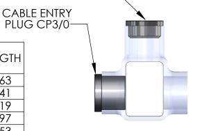
**WIRE ENTRY POINT** WIRE RANGE: 3/0 - #6AWG PRE-FILLED W/ OXIDE INHIBITOR
