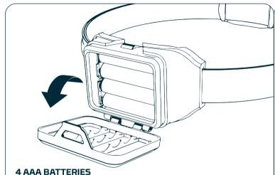
Open the battery compartment, remove old batteries and dispose of properly. Insert 4 new AAA batteries, making sure the negative ( - ) end of the battery faces the spring.
