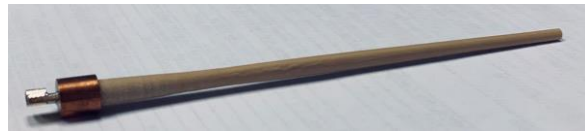
Figure 6: Cylindrically shaped dielectric rod (length = 10 cm, operating freq. = 28 GHz). Approximately 20dBi gain.
