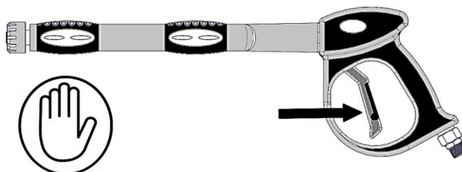
3. Check that the pressure indicated on the pressure gauge matches the value on the data plate and in the technical data. Also check that when the trigger is released the pressure shown on the gauge returns to zero.
