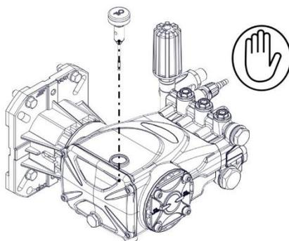
9. If applicable check the oil level in the gearbox using the sight glass on side of gearbox. Make sure the oil is level with the indicator on the sight glass. If oil reservoir needs replenishing only use oil of a type as listed in the data sheet in this instruction manual.
