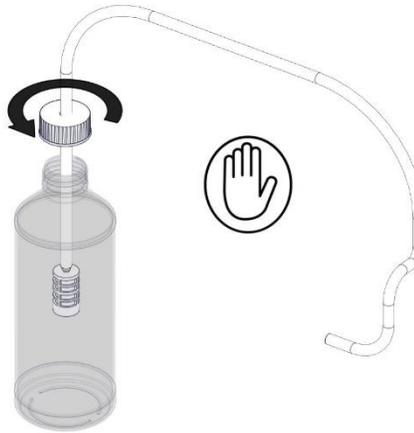
3. Open the chemical injector by turning the knob anti-clockwise until the desired affect is reached. When the trigger is pulled, water mixed with detergent will be sprayed.
