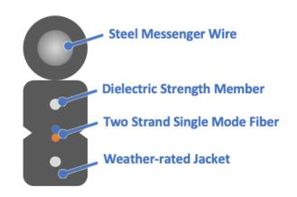
S2I-2F-L-BK fiber optic cable is constructed with two internal tight buffered single mode fibers, dielectric strength members, an integrated galvanized steel messenger wire, and an overall outdoor-rated LSZH jacket. The cable is designed for aerial, underground direct burial and FTTH (fiber-to-the-home / fiber-to-the business) applications.
