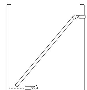
7. Insert the BRACE POST (F) into the bottom BRACE CUP (A) of the LINE POST (E). Secure the BRACE POST (F) by drilling a SELF-TAPPING SCREW (H) through both BRACE CUPS (A) and BRACE POST (E). Once secured, tighten the CARRIAGE BOLT (C) on both BRACE BANDS (B).
