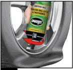
Turn can upside down and screw plastic nozzle clockwise onto tire valve.
