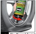
Allow 30 seconds for can to discharge fully. Unscrew nozzle when empty.
