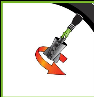
**6** Reinstall valve core.
