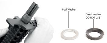
NOTE: Crush washers are NOT recommened as they do not crush uniformly and WILL cause improper mounting and baffle strikes. Silencerco recommends a peel washer if any clocking of the mount is required
