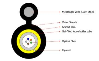
OSPFiber<sup>™</sup> Flgure-8 fiber optic cable is constructed as a gel-filled loose-tube cable with an integrated galvanized steel messenger wire, and an overall outdoor-rated LSZH jacket. The cable is designed for aerial, underground direct burial and FTTH (fiber-to-the-home / fiber-to-the business) applications.
